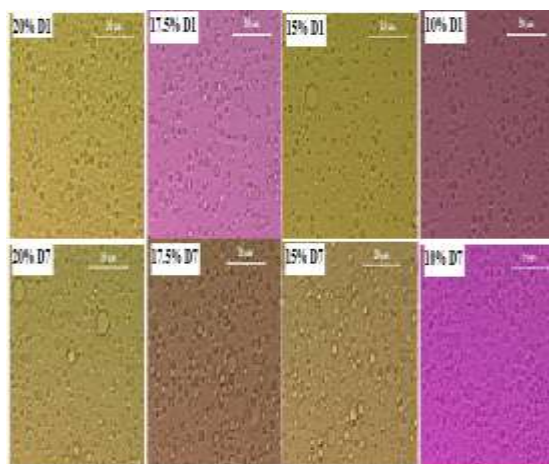
Fig. 3: Microscopy images of ASY gum emulsion samples after one day (D1) and seven days (D7) of incubation at 45°C with varying IPM oil concentrations: 20%, 17.5%, 15%, and 10%
