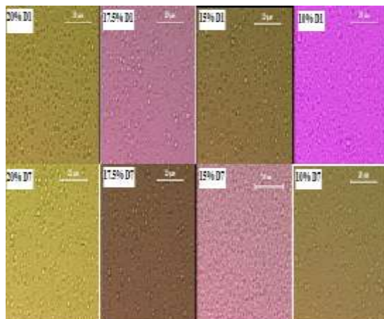
Fig. 4: Microscopy images of ATR gum emulsion samples after one day (D1) and seven days (D7) of incubation at 45°C with varying IPM oil concentrations: 20%, 17.5%, 15%, and 10%.
