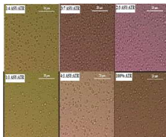
Fig. 5: After one day of incubation at 45°C, microscopy images of ASY and ATR gum blend emulsions (1:4, 3:7, 2:3, 1:1, and 4:1 ASY: ATR) with 20% IPM oil concentration were obtained.
