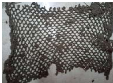
Figure 22. The second sample after one month of burial
