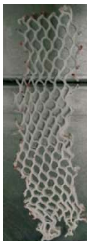
Figure 27. Sample of PLA mesh fabric after one week
