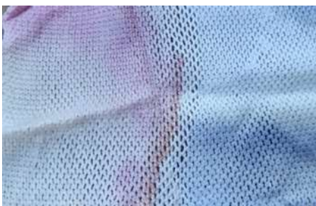
Figure 20. The sample after 3 days with purple spots
