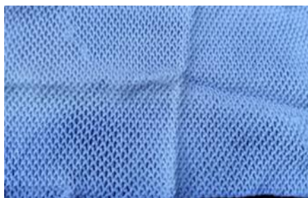
Figure 14. Produced sample of PLA saturated with indicator of red cabbage
