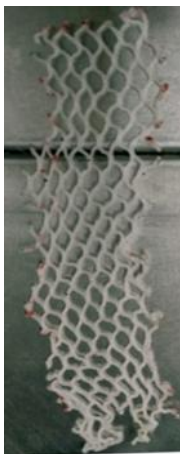
Figure 27. Sample of PLA mesh fabric after one week
