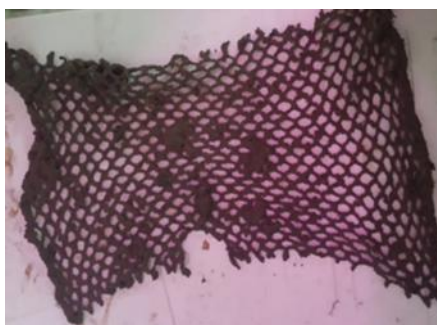
Figure 23. The second sample after two months of burial
