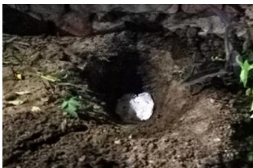
Figure 6. Buried mesh samples of PLA in soil
