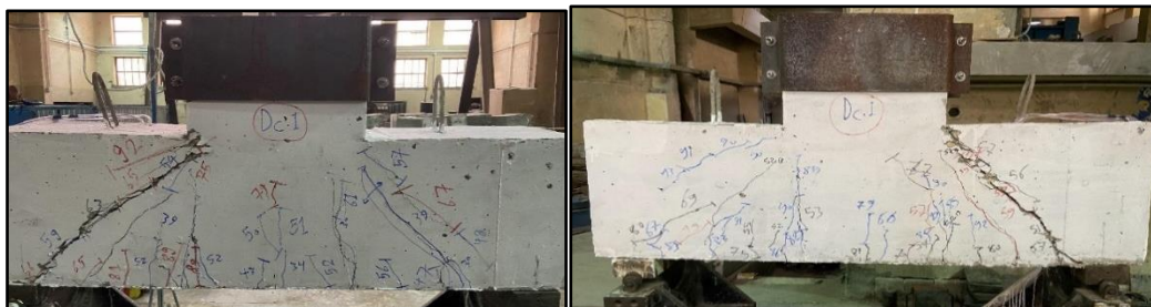
Fig 10. Crack patterns for specimens (DC1) with no eccentricity
