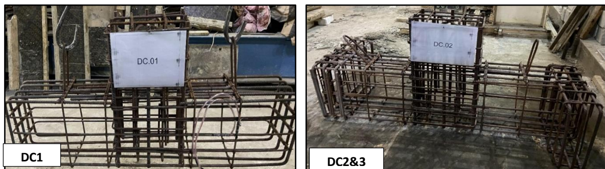
Fig 6. Reinforcement cage for RC corbels DC1, DC2 and DC3
