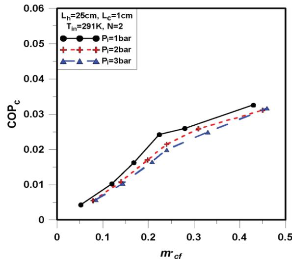
Fig. 5: Effect of cold mass fraction ( $m_{cf}$ ) on the  $COP_c$  at different values of inlet pressure, 2 nozzles and  $L_h = 25$  cm.
