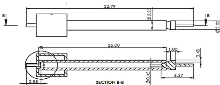
Fig. 1: Dimensional components of vortex tube (cm).
