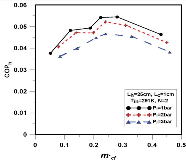
Fig. 6: Effect of cold mass fraction ( $m_{cf}$ ) on the  $COP_h$  at different values of inlet pressure, 2 nozzles and  $L_h = 25\text{cm}$ .
