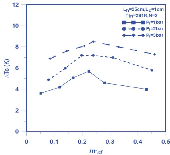
Fig. 3: Effect of cold mass fraction ( $m_{cf}$ ) on the cold temperature difference at different values of inlet pressure, 2 nozzles and  $L_h = 25$  cm.
