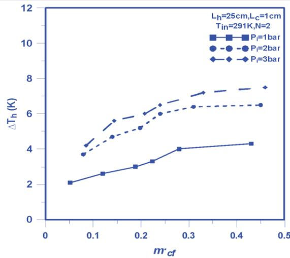
Fig. 4: Effect of cold mass fraction ( $m_{cf}$ ) on the hot temperature difference at different values of inlet pressure, 2 nozzles and  $L_h = 25$  cm.
