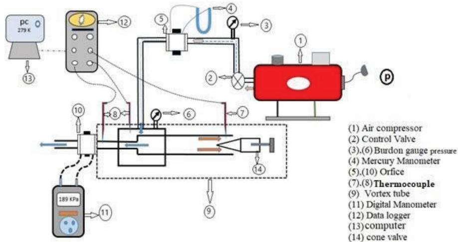
Fig. 2: Layout of experimental setup.
