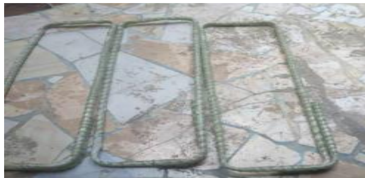
Fig. 3. Surface characteristics G-F-R-P bars.
