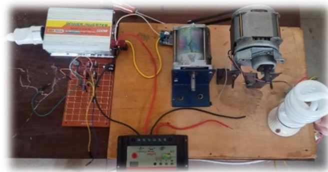
Fig.25. DC Microgrid system connection.
