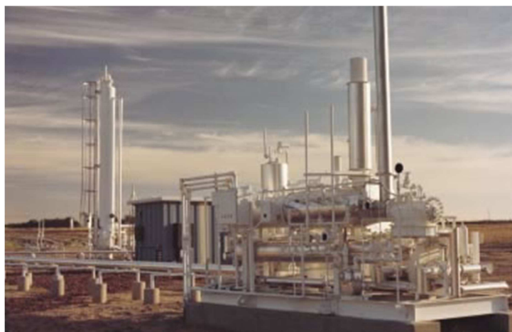
Figure 4: Direct Fired Glycol Reboiler [39]
