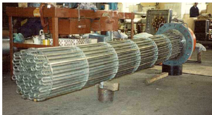
Figure 3: Electrical Glycol Reboiler Bundle [31]
