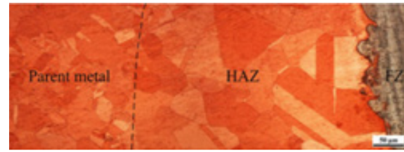
Fig. 22: Microstructures of the heat-affected zone at the copper side and at the interface between copper and the fusion zone Chen et al. [22] .
