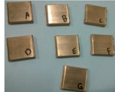
Fig. 5: 30*30*5 Samples before cutting
