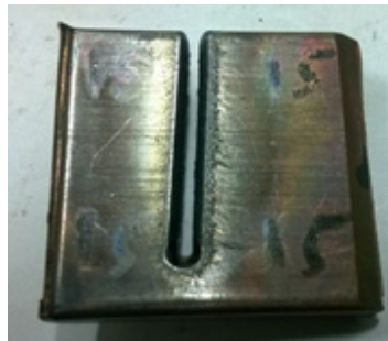
Fig. 4-B: Top spatter on the upper surface of the plate
