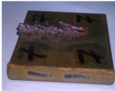
Fig. 4-A: Adhering low speed dross to the bottom of the plate
