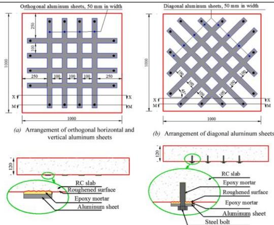
Fig. 4. Application of aluminum sheet for improve punching [82].
