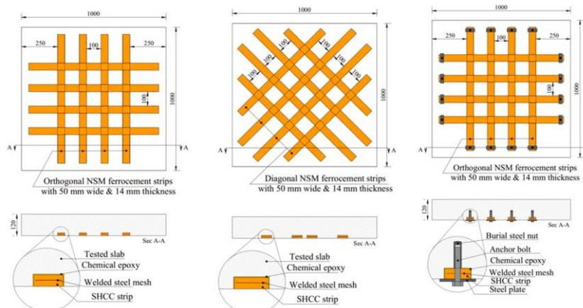
Fig. 1. Anchored and epoxied ferrocement strips used for strengthening punching [80]
