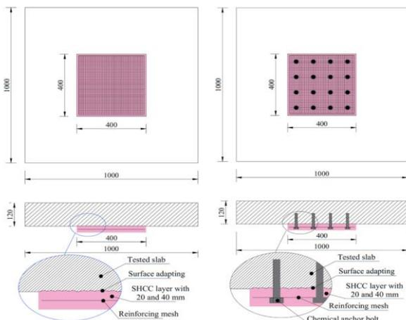
Fig. 2. Drop panels used for strengthening punching [81]
