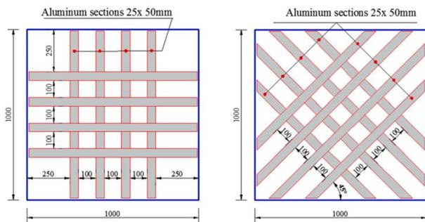
Fig. 5. Utilizing of aluminum sections for improve shear punching [83].
