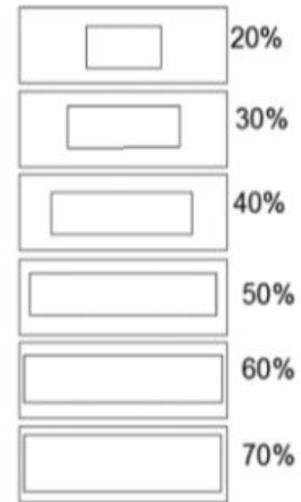
**Figure (2):** Window-to-Wall Ratio (WWR) and the position of the window on the façade
