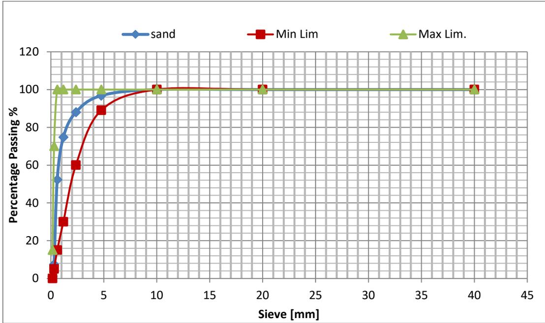
Fig.1. Sieve analysis of fine aggregate
