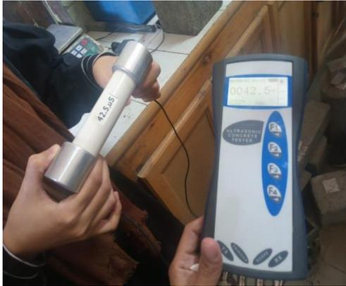
Fig.7. Calibrating the ultrasonic device before starting
