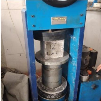
Fig. 4. Compression strength test
