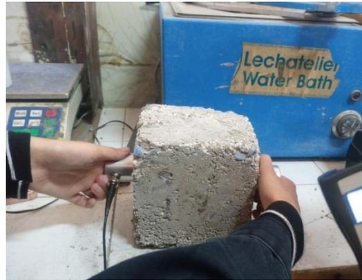
Fig.8. Ultrasonic-pulse waves through Polystyrene-concrete sample
