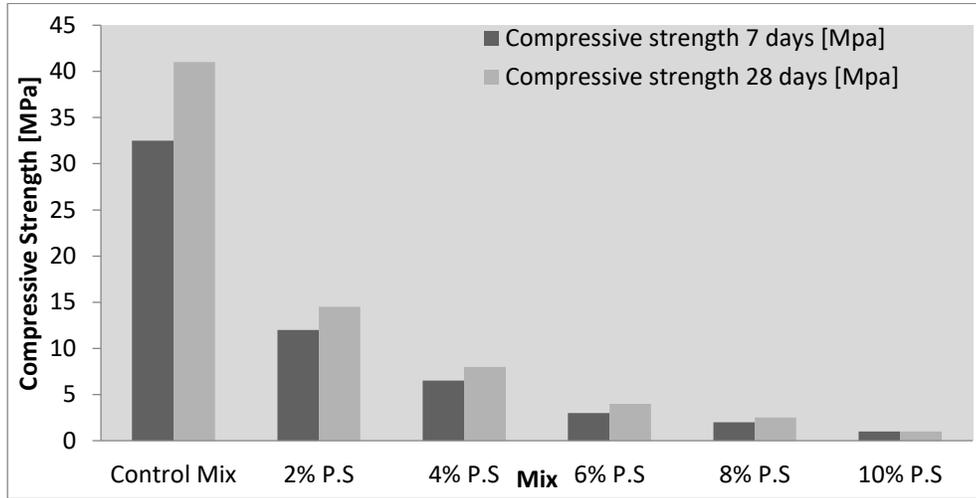
Fig.9. compressive strength results
