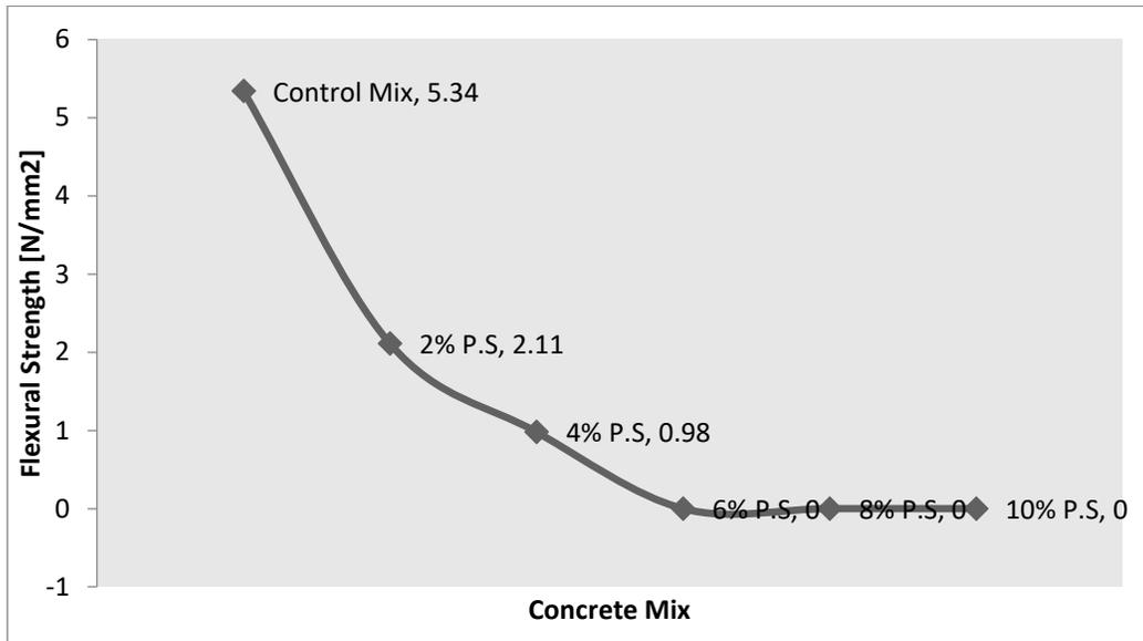
Fig. 10. Flexural Strength test results
