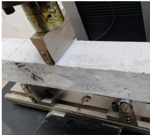
Fig. 6 flexural strength test loading
