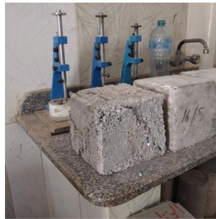
Fig. 5. specimens after failure.
