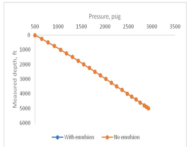
**Figure 5** Pressure traverse for no water cut with and without emulsion correction
