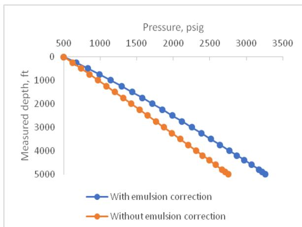
**Figure 7** Pressure traverse for water cut of 50% with and without emulsion correction
