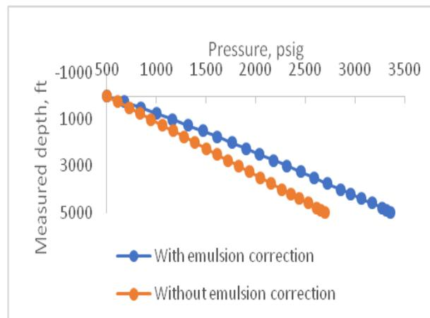
**Figure 8** Pressure traverse for water cut of 75% with and without emulsion correction
