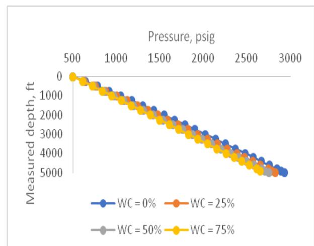
Figure 3 Pressure profile along the wellbore with no emulsion viscosity
