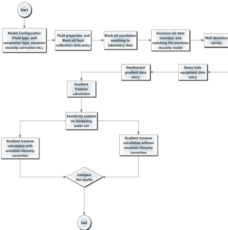
Figure 1 Simulation workflow
