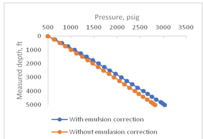
**Figure 6** Pressure traverse for water cut of 25% with and without emulsion correction.
