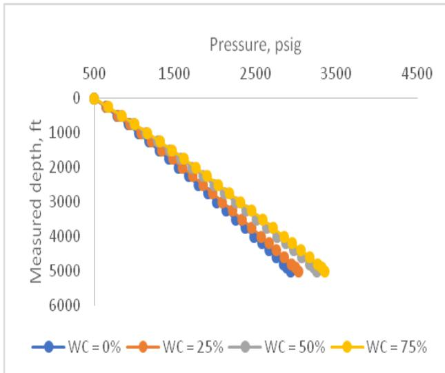
**Figure 4** Pressure profile along the wellbore with emulsion model correction
