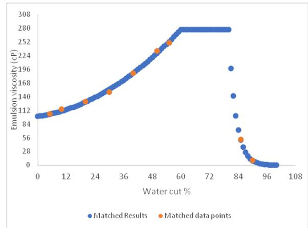
Figure 2 Experimental and simulated emulsion viscosity
