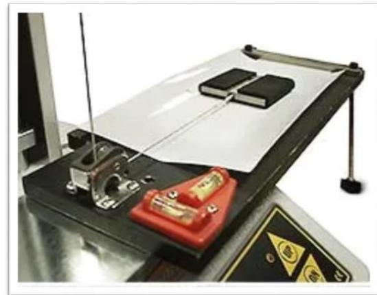
Figure 6. shows the COF measurements on mechanical testing machine (photography be researcher, NRC)
