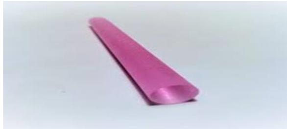
Fig.13. real image of ND-YAG rod.
