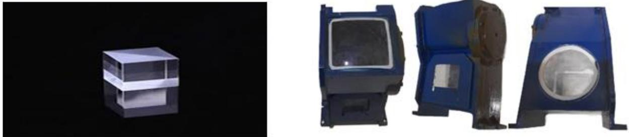
Fig.31, 32. the two perpendicular prisms were placed from the base and different view chassis of dichroic beam splitter charged with nitrogen
