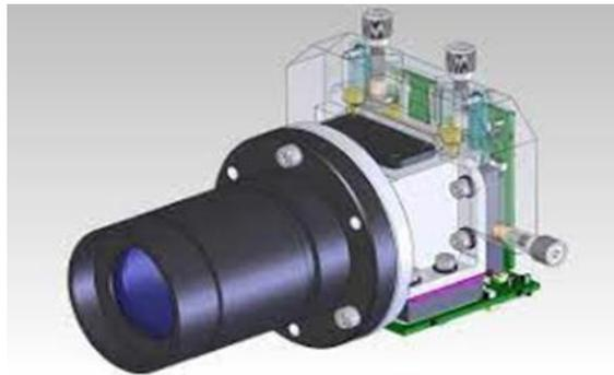
Fig.35. the 3D design of a proposed camera with optical system
