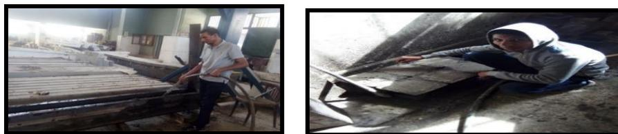
FIGURE 3: Concrete Pouring of Test Specimens
