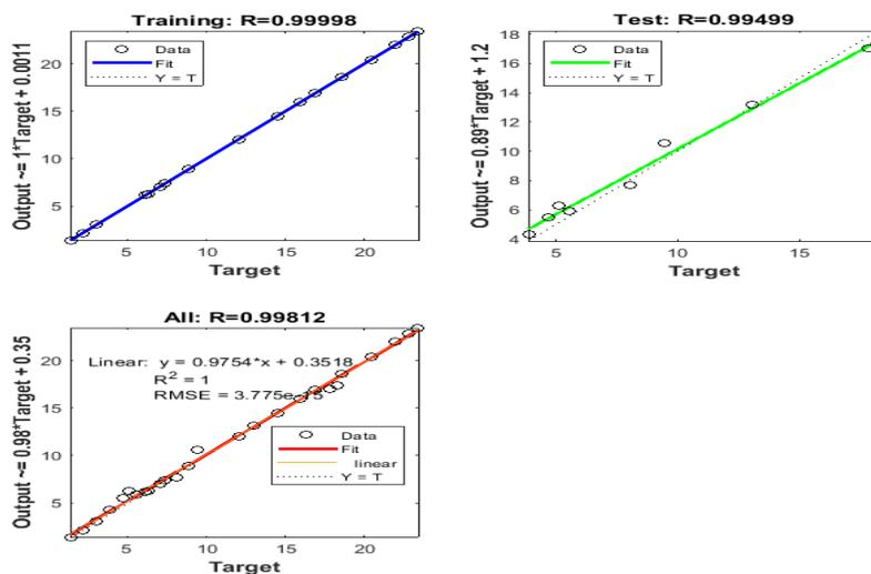
**Figure 9:** Error regression residuals plot for modelling compressive strength using RBF
