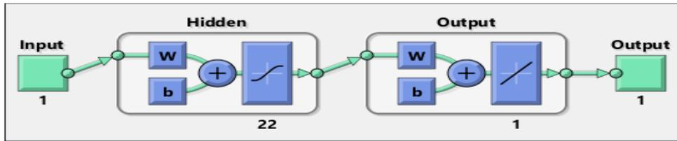
Figure 1: MLFFNN architecture for modelling compressive strength
