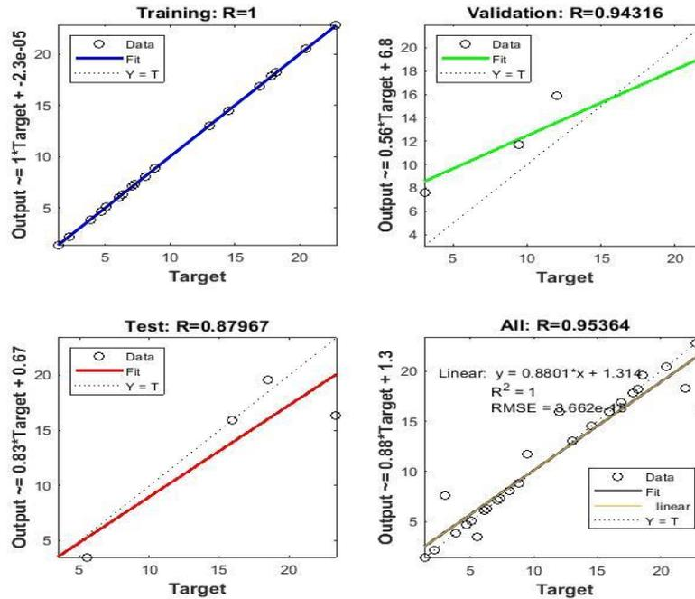
**Figure 4:** MLFFNN error regression residuals plot for modelling compressive strength
