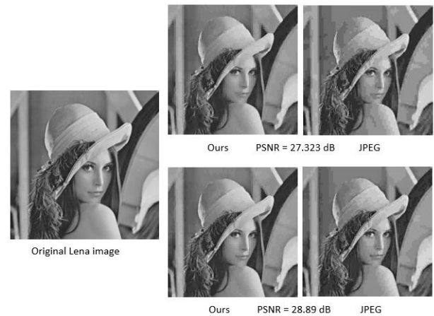
Figure 8. Original and Reconstructed Lena Images from Proposed Method and JPEG
