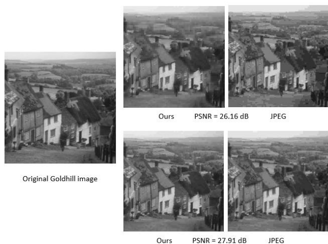
Figure 12. Original and Reconstructed Goldhill Images from Proposed Method and JPEG
