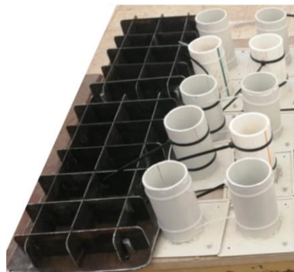
Figure 2. Compressive strength and tensile strength test moulds .
