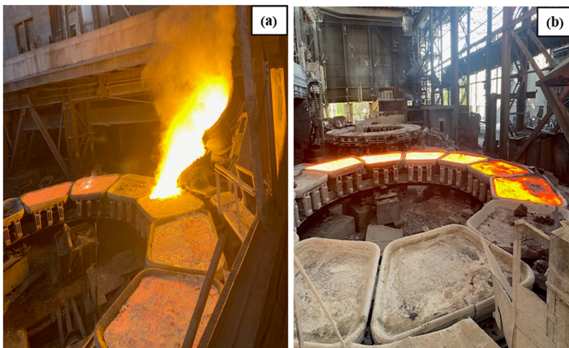
Figure 1: The casting process of FeSiMg alloy, (a) during pouring, (b) after complete pouring.
