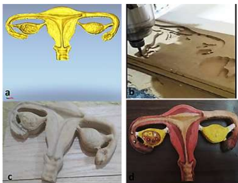
Fig 2. a- showing stl file format for production of genital system. b- showing CNC router during manufacturing genital system- c- showing produced wood engraved genital system. d- showing genital system after coloration
