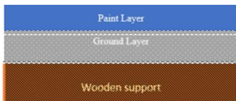
Figure 7. The layered composition of icon understudy
