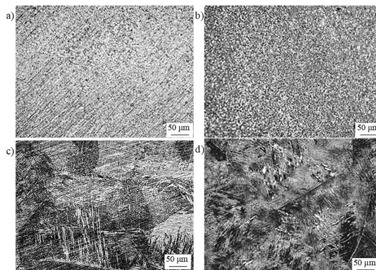
**Fig. 4** OM of the as-forged (a,b) and as-cast (c,d); Ti64 and Ti67 alloy samples, respectively, from the left side. License from [12].
