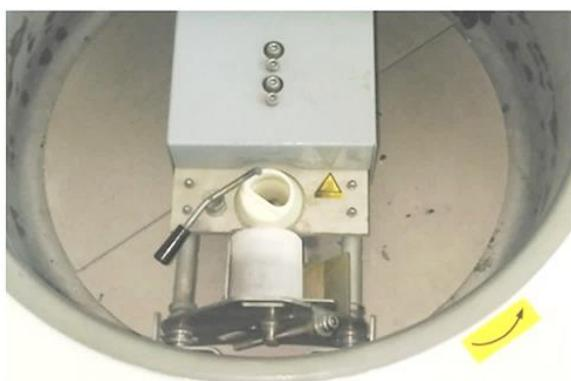
**Fig. 2** Casting setup using a vacuum centrifugal casting machine.
