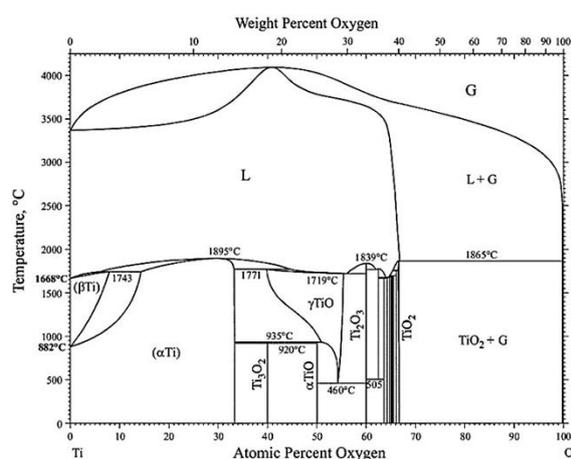
**Fig. 1** Ti-O phase diagram [1].
