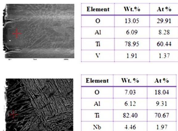
**Fig. 10** EDX point analysis in the oxygen diffusion layer of the forged Ti64 (top) and Ti67 (bottom) samples oxidized at 1373 K (1100 °C) [License from 12].
