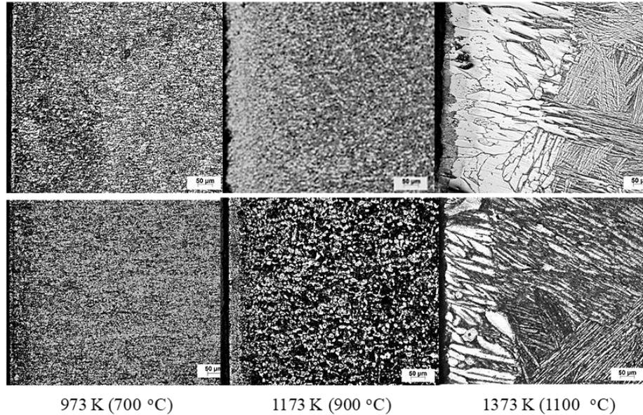
**Fig. 7** Optical micrographs of the cross section of the forged samples Ti64 (top) and Ti67 (bottom), after oxidation at different temperatures, License from [12].
