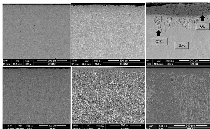
**Fig. 5** FEM compositional image of the oxidized –forged samples, Ti64 (top) and Ti67 (bottom) at 973 K (700 °C), 1173 K (900 °C) and 1373 K (1100 °C) respectively from the left side. The oxide layer, oxygen diffusion layer, and base metal were denoted as OL, ODL, and BM, respectively.
