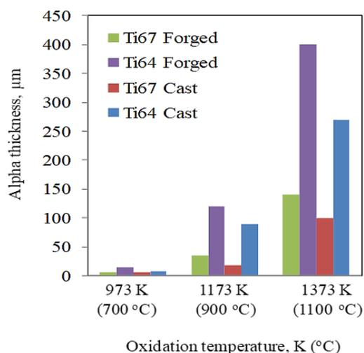
**Fig. 9** Maximum thickness of alpha case in the oxidized samples from the micrographs of Figs. 7 & 8
