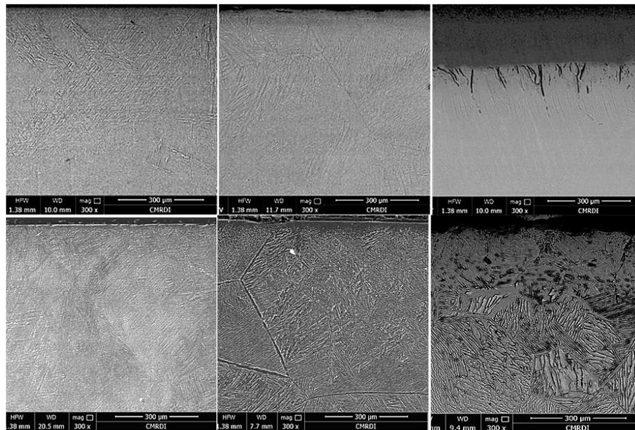
**Fig. 6** FEM compositional image of the oxidized –cast samples Ti64 (top) and Ti67 (bottom) at 973 K (700 °C), 1173 K (900 °C) and 1373 K (1100 °C) respectively from the left side. The oxide layer, oxygen diffusion layer, and base metal were denoted as OL, ODL, and BM, respectively
