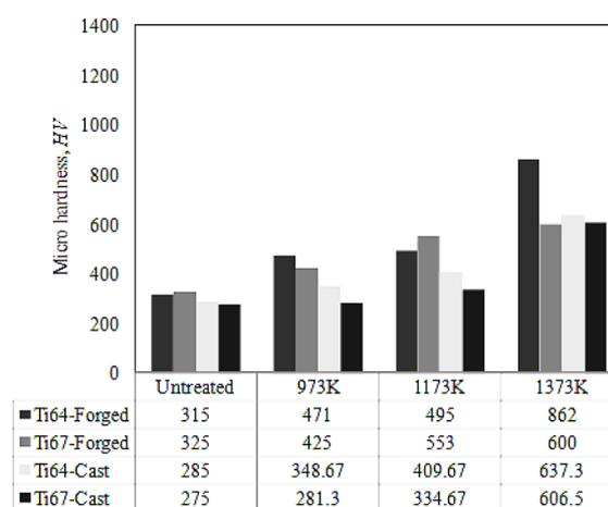
**Fig. 11** Microhardness of the untreated and oxidized samples just below the oxide layer.
