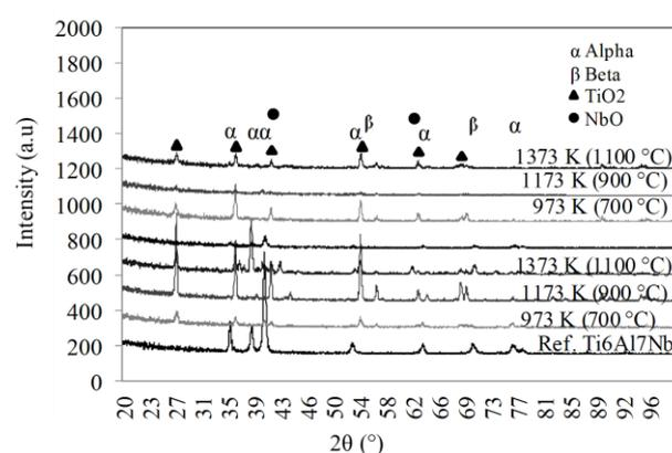
**Fig. 3** XRD patterns of the as-received and oxidized Ti64 and Ti67 samples, License from [12].
