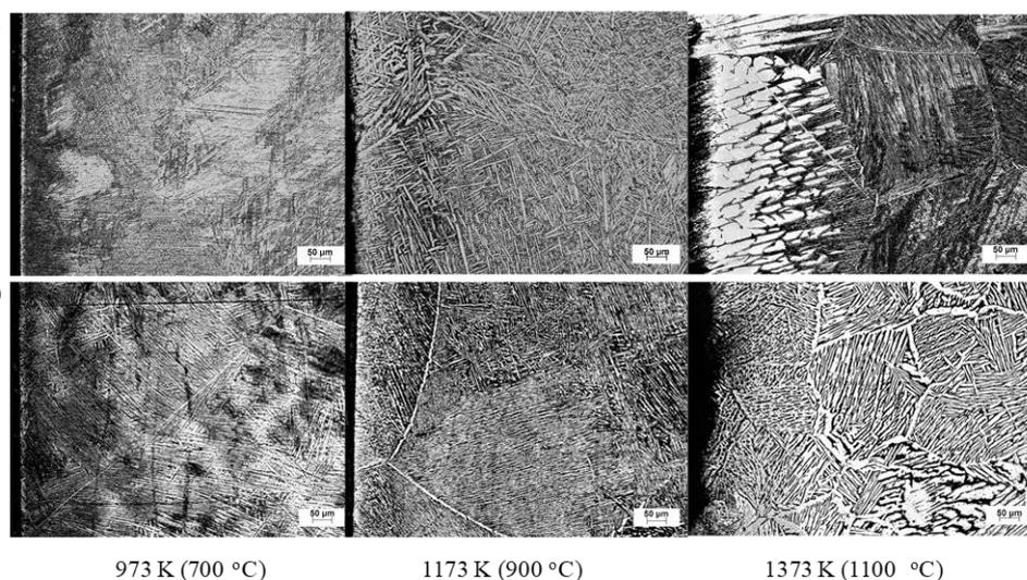
**Fig. 8** Optical micrographs of the cross section of the cast samples Ti64 (top) and Ti67 (bottom) after oxidation at different temperatures. License from [12].
