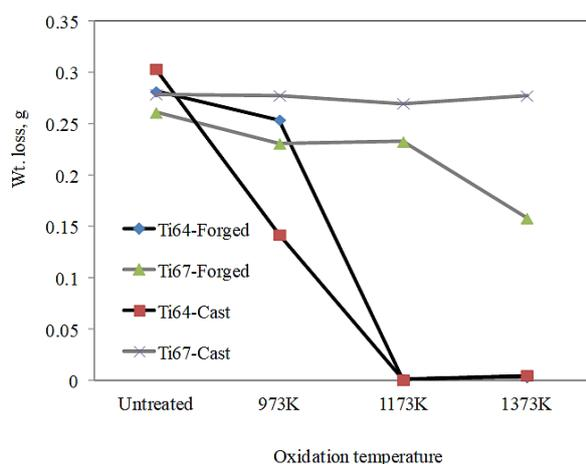
**Fig. 12** Wear resistance of the untreated and oxidized forged samples.
