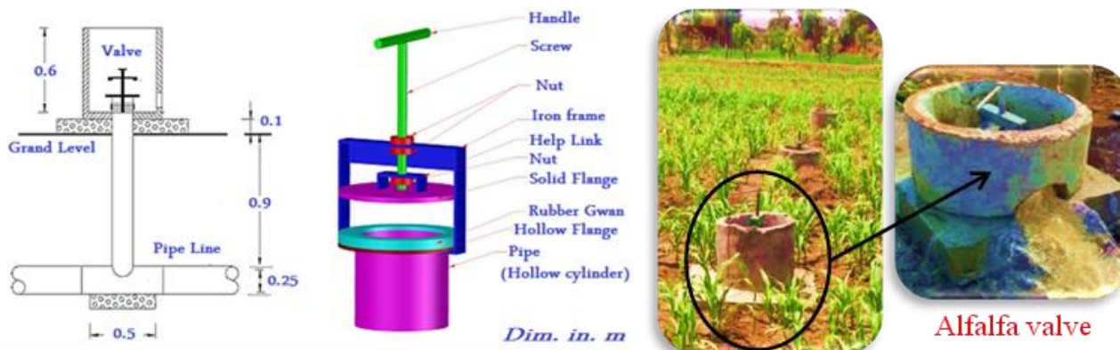
Fig. 5. A schematic diagram showing buried pipes dimensions
