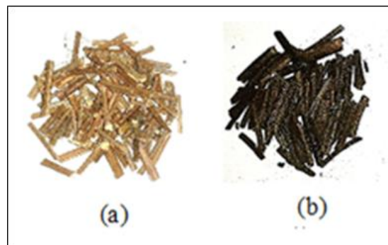
Fig. 2: Effect of torrefaction process on the color of cotton stalk (a) before torrefaction and (b) After torrefaction process
