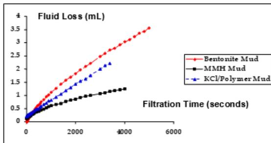
**Figure 10** Fluid loss variation based on mud type
