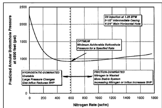
Figure 15 There is optimum nitrogen rate to control the bottom hole pressure and the wellbore stability [44]
