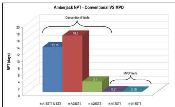
Figure 13 Less non-productive time (NPT) for MPD compared to conventional drilling [42]
