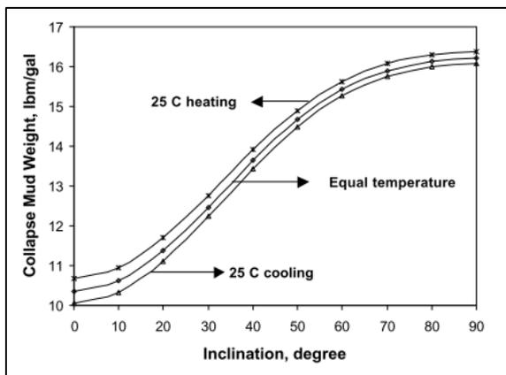
**Figure 6** Thermal impacts on collapse mud densities for inclined boreholes [27]
