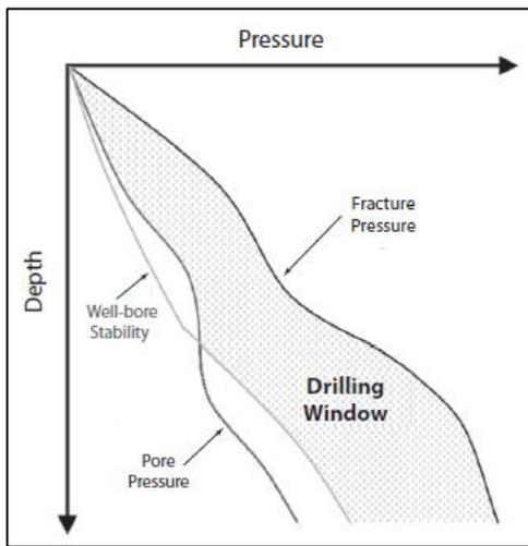
Figure 12 MPD good choice for narrow drilling window to avoid fracture formation and wellbore instability [40]
