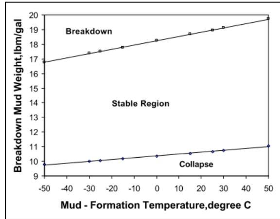
**Figure 7** Impact of temperature variations on essential mud weights for vertical boreholes [27]
