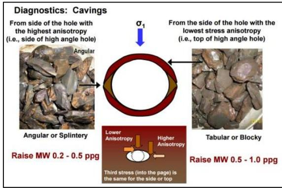
Figure 2 showing the effect of the MW on shape caving and wellbore stability [26]
