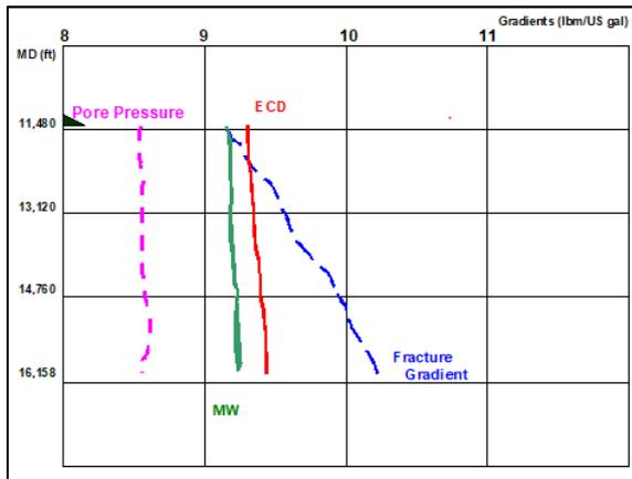
Figure 3 Example of drilling pressure window, presenting possibility of fracture the formation during circulation due to the higher ECD
