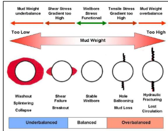
Figure 4 Formation pressures on the wellbore are kept in check with mud weight. Because the formation pressures are different at different depths, the average density of the mud may cause problems at some depths[29]
