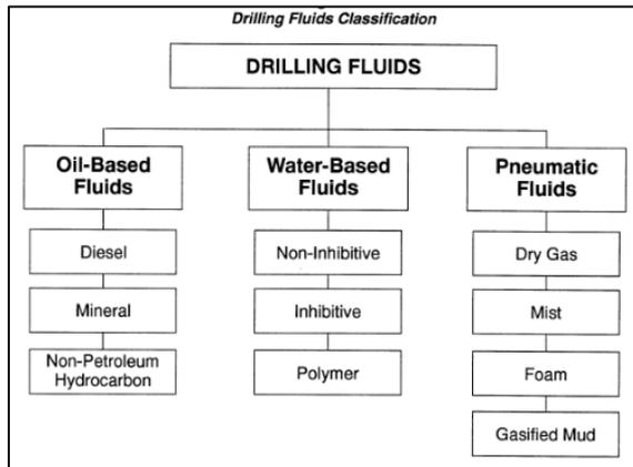
**Figure 1** Drilling Fluid Classification [11]
