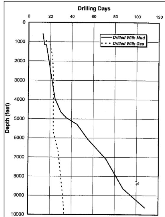
Figure 14 UBD can improve drilling rate of penetration (ROP) and total days of drilling [44]
