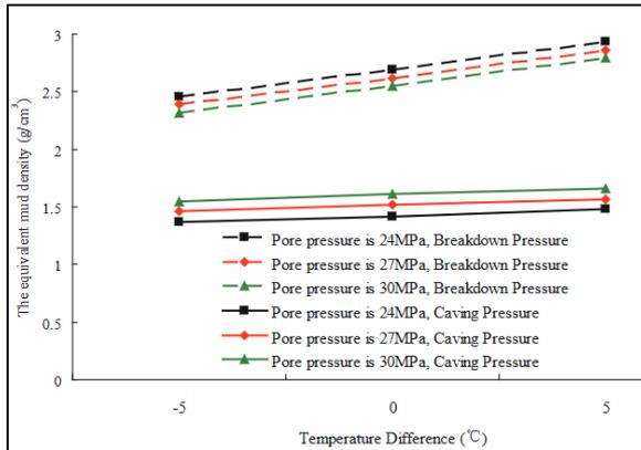
**Figure 9** The Impact of Temperature Variation on the Safety Mud Density Window in Relation to Varying Borehole Rock Pore Pressure [31]
