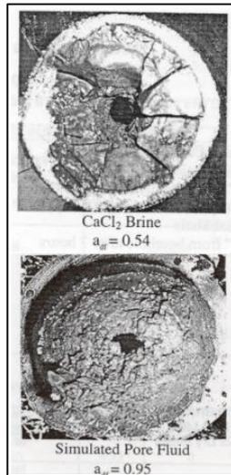
**Figure 5** Shale samples from the Gulf of Mexico subjected different drilling fluids under conditions of zero hydraulic differential pressure [4]
