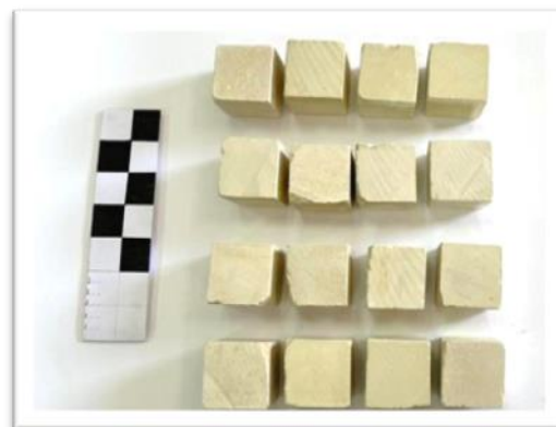
Figure 1 : Illustrates the preparation and processing of experimental limestone cubes prior to the consolidation treatment
