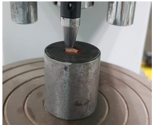
Fig. 4. Sample mounted onto Vickers hardness tester.
