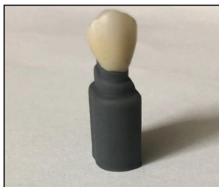
Figure (1): Zirconia crown seated on 3D printed resin die
