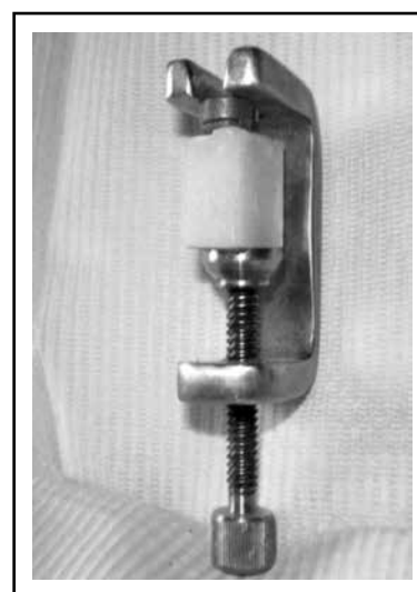
Fig. (1) Holder with block Upper part has U shape space Specimens The lower part has screw
