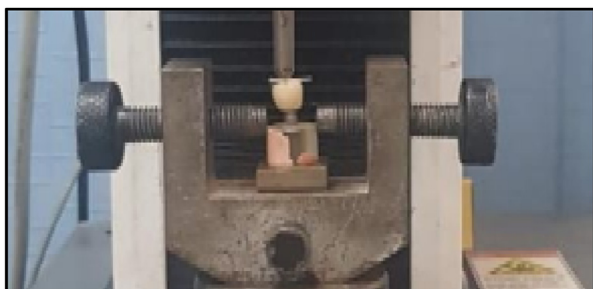
Fig. 3. Sample fixed on the universal testing machine.
