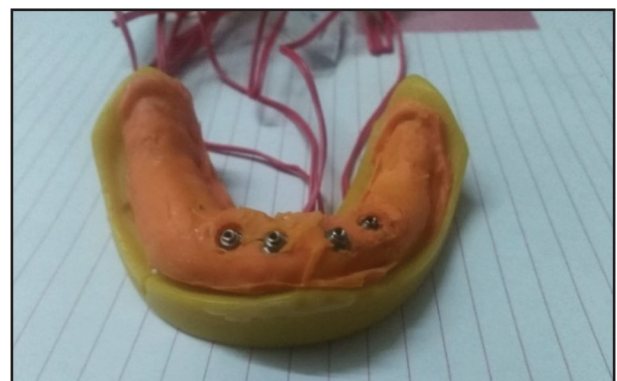
Figure (4): Strain gauge installed
