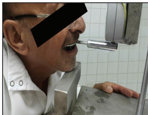
Figure (8) Digital force-meter device for retention evaluation.
