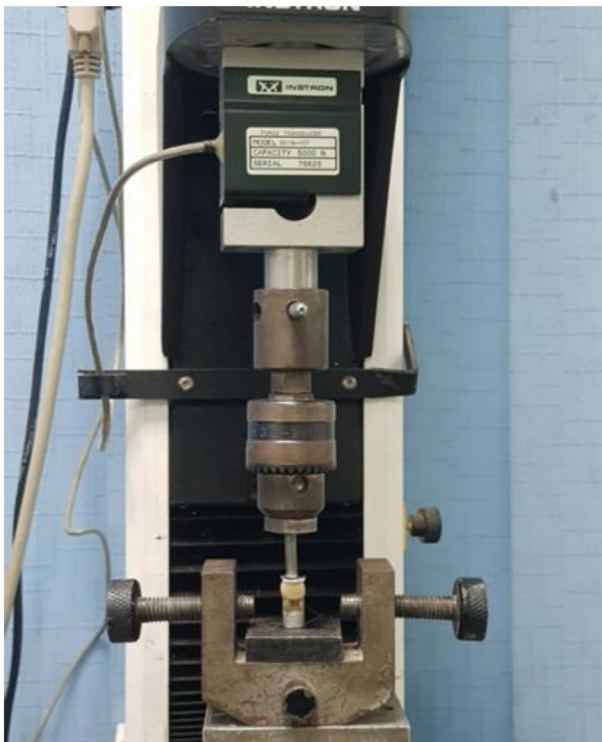
Fig. 2. Sample in universal testing machine for fracture resistance test.
