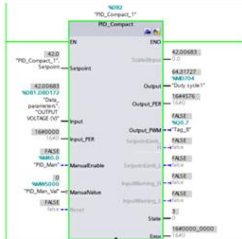
Fig. 9: Block diagram of PID compact
