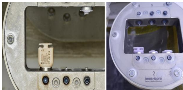
(Figure 2 ): (A)Milled LiSi T specimens attached to support structure.(B)Milled LiSi E specimens before support removal.
