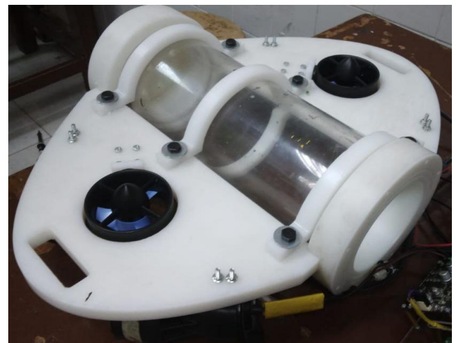
Figure 17: Realistic Assembly of Final ROV Configuration.
