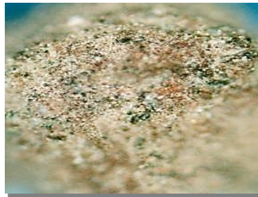
Fig. 17 Air cold slag under reflected light, magnification \times 50 .
