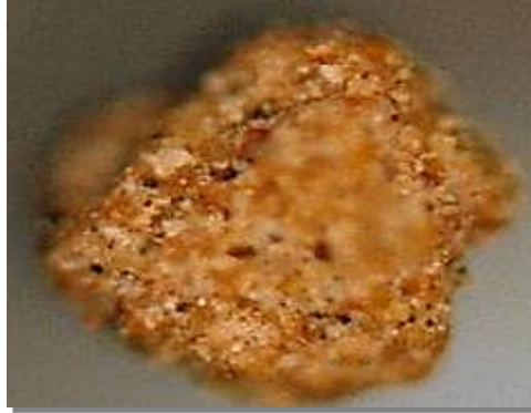
Fig. 8 Fatty clay particles under reflected light, magnification \times 100 .
