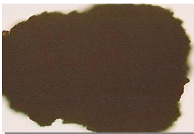
Fig. 2 Clinker particle under transparent light, magnification \times 50 .
