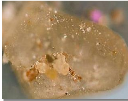
Fig. 10 Sandy clay particle under cross-reflected light, magnification \times 100 .
