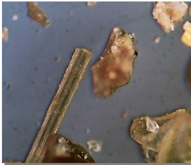
Fig. 21 Accumulated water cooled slag particles under cross reflected light, magnification \times 50 .
