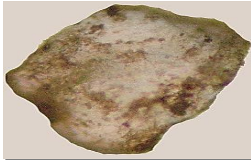
Fig. 6 Fatty clay particles under reflected light, magnification \times 50 .
