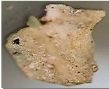
Fig. 19 Air cooled slag low ferric under cross transparent light, magnification \times 50 .
