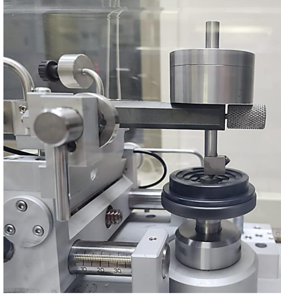
Fig. 3 CSM pin-on-disc tribometer for wear testing.
