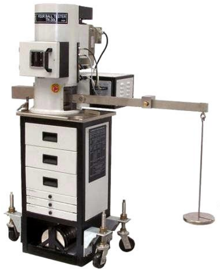
Fig. 5 Four Ball Tester.
