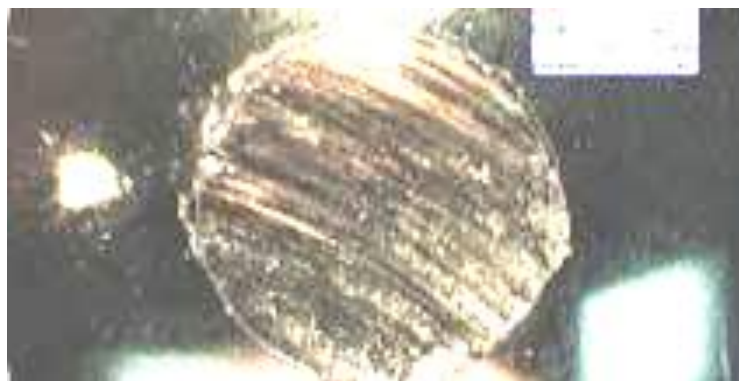
Fig. 6 Example of Scar Diameter.
