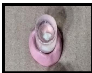
Fig. (3): Embedding of specimens in epoxy resin with their buccal surface facing upwards.
