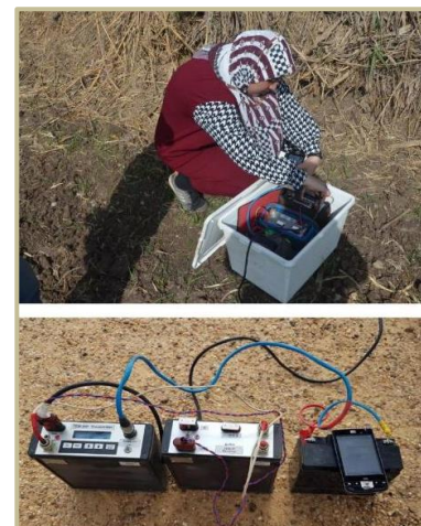
Figure 6 . Field setup for Time-Domain Electromagnetic (TDEM) data acquisition. (Top) Configuring the receiver and connecting the loop. (Bottom) AIE-2 Measuring System, including a power source connected to the transmitter, and loop connections for signal generation. A phone-like unit controls the survey parameters and operation.
