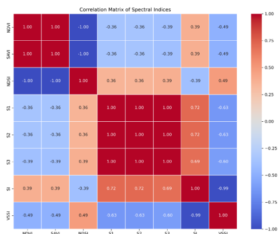
Figure 8 Correlation matrix showing relationships between vegetation, brightness, and composite salinity indices used to assess coastal salinization. Strong contrasts highlight complementary index behavior.
