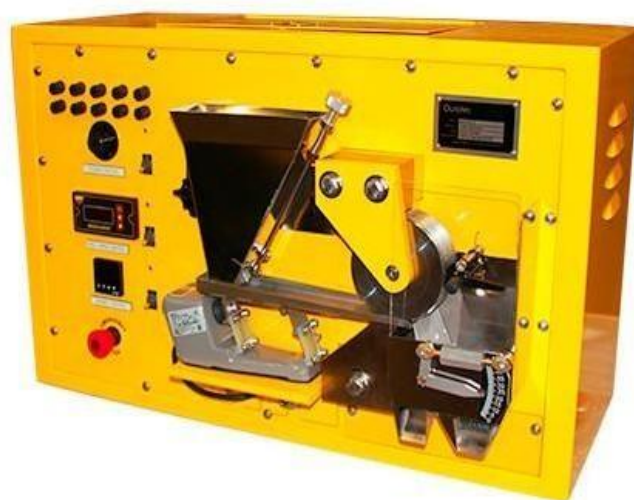
Figure (5): Shows the Laboratory high intensity induced roll magnetic separator.
