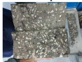
c. Splitting for FA 450-A0.35 samples
