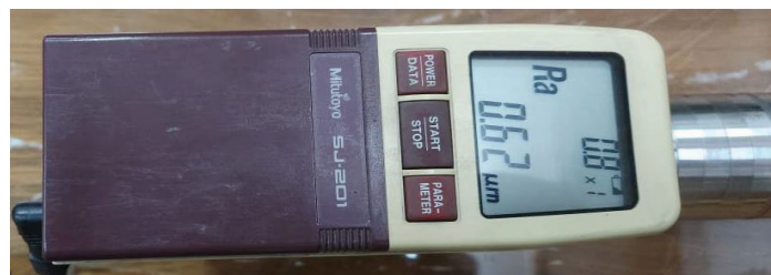
Fig. 5: Setting Up of SJ-201 Mitutoyo Surf Test to Measure the Surface Roughness for the Burnished Workpieces.
