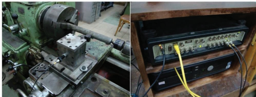
Fig. 7: Setup of Vibration Measurement Equipment including, (a) the 4514 Accelerometer, and (b) the 2560 C Signal Analyzer.
