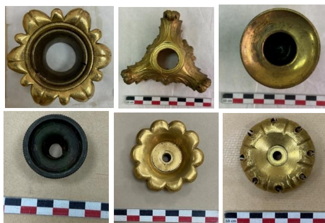
Fig. 21. Candelabra parts after treatment and protection with 0.5% BTA + (5mg) \text{TiO}_2 .
