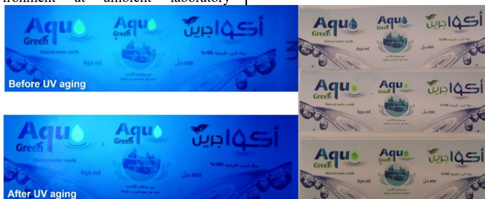
Figure 7 eyes visualization of printed packaging labels with FL inks before and after UV aging under normal and UV-light
