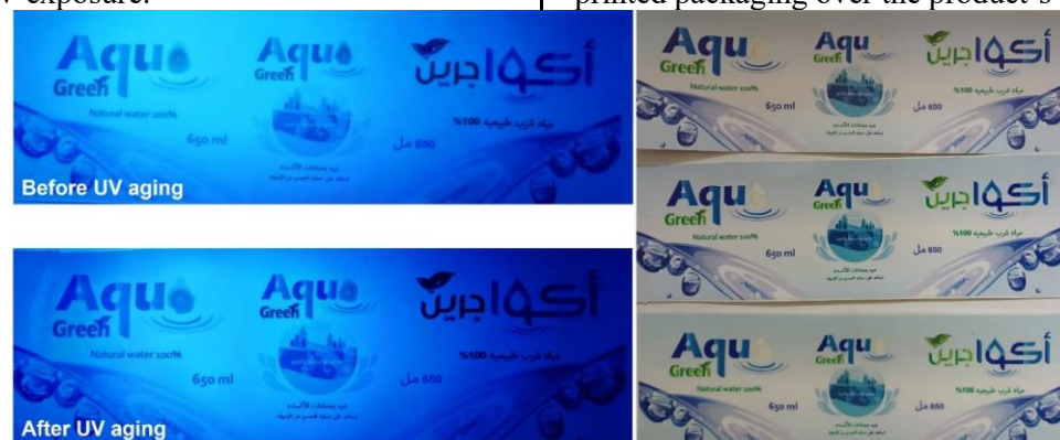
Figure 8 eyes visualization of printed packaging labels with PC inks before and after UV aging under normal and UV-light
