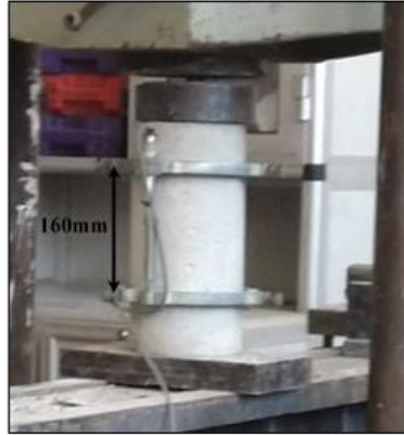
Fig. 6: Test Setup for Investigating Young's Modulus
