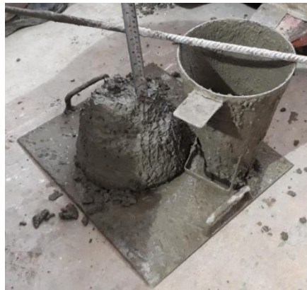
Fig. 2: The Performed Slump Test
