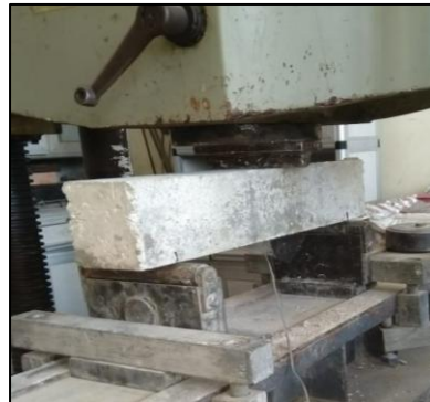
Fig. 4: Test Setup for Flexural Strength
