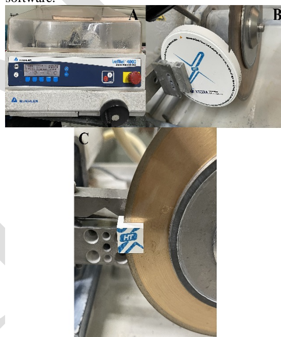
Figure (1): Cutting of zirconia specimens using slow speed saw microtome
