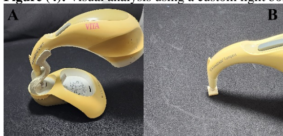
Figure (5): Instrumental analysis using vita easyshade, All Specimens were measured by holding the probe tip at 90° to the surface of each specimen at the center of the specimens and the reading was repeated 3 times for each specimen
